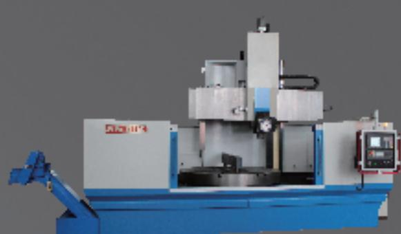
▲ Single Column Vertical Lathe-CNC
