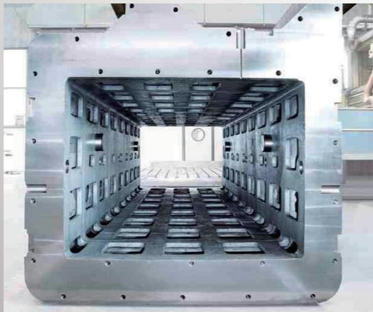
The two ground rails in front of the column check the position of the spindle box and ensure the steadiness of spindle's vertical movements. The column is equipped with preload precision double-nut ball screws, and servo motor drives the vertical travels of the spindle box.
