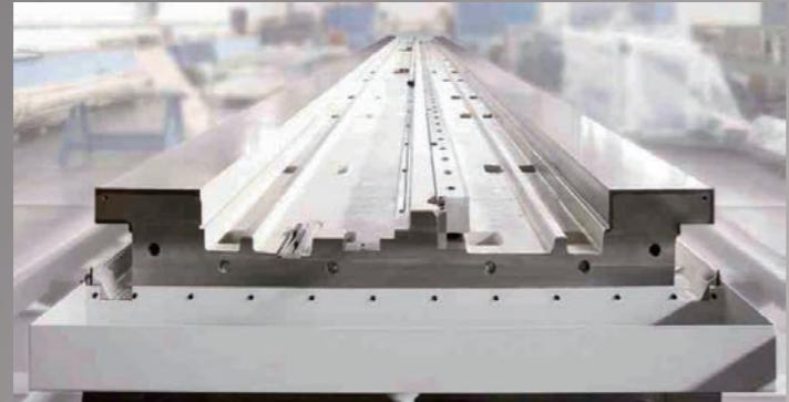
The machine bed is built of resin, wood former with reasonable structure and rigidity. It guarantees a sound base and steady machine, also ensures a stable column when it's in motion. The machine is equipped with top quality dent surface racks which are imported from overseas, and two preload co-drive gears that ensures the accuracy of the X axis.
