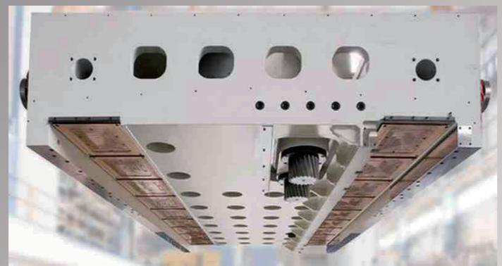
Built with top quality castings, resin and wood former, the sliding carriage possesses sufficient intensity. It connects to the machine bed with two wide guide ways. The single guide way serves as main positioning with the support from other double guide ways to maintain the stability and linearity of column in motion on machine bed.
